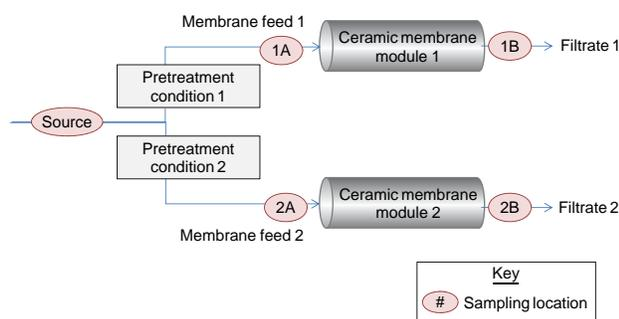
**Figure 2** | DWU pilot test sample locations.
