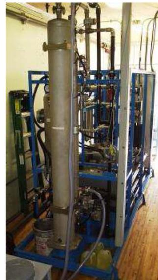
**Figure 3** | City of Rifle ceramic membrane pilot system.
