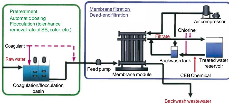
Figure 4 | City of Rifle ceramic membrane pilot system process flow diagram.
