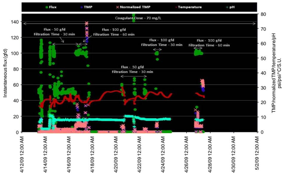
**Figure 6** | DWU ceramic membrane pilot test results for spent filter backwash water.
