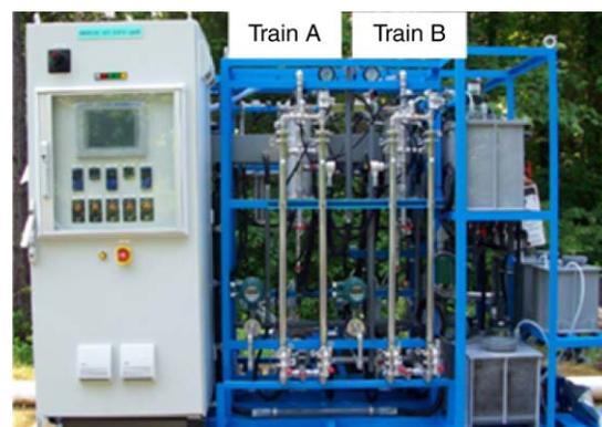
Figure 1 | DWU ceramic membrane pilot system.
