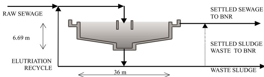
**Figure 1** Schematic presentation of the full-scale APT configuration
