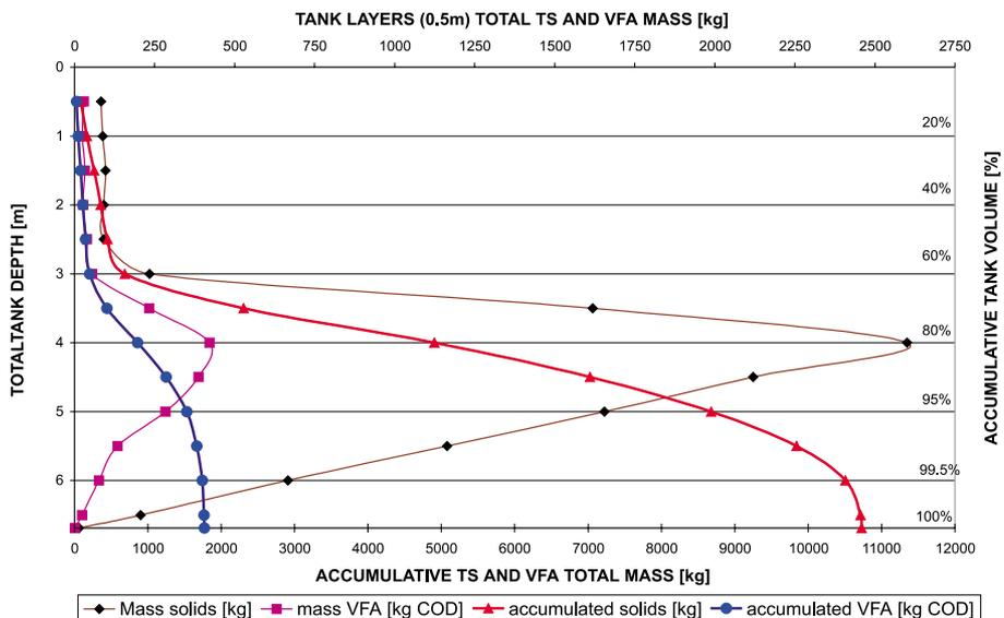
**Figure 2** TS and VFA mass and cumulative mass profiles, high sludge blanket APT
