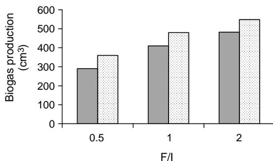
**Figure 6** Cumulative biogas production vs. F/I ratio
