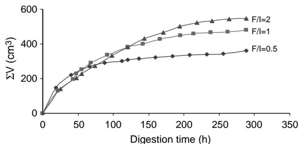
**Figure 5** Biogas produced in the tests at different F/I with sonicated sludge
