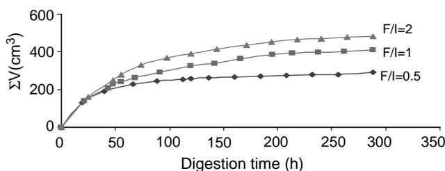
**Figure 4** Cumulative biogas production at different  $F/I$  with untreated sludge
