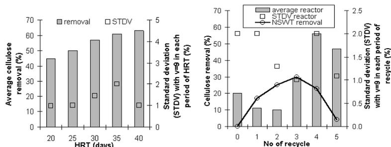
**Figure 3** Average cellulose removal in R-1 at several HRT. Average cellulose removal in R-2 at (0): AHT coupled with methane fermentation and (1–5): AHT coupled with methane fermentation with NSWT and cellulose removal in NSWT
