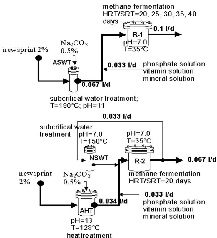
**Figure 1** Pretreatments for newsprint waste. Alkaline subcritical-water treatment (ASWT) and alkaline heat treatment (AHT) combined with neutral subcritical-water treatment (NSWT)
