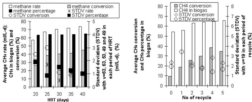
**Figure 2** Average methane rate, methane in biogas, and conversion eff. in R-1 at several HRT. Average methane conversion eff. and methane in biogas in R-2 at (0): AHT coupled with methane fermentation and (1–5): AHT coupled with methane fermentation with NSWT
