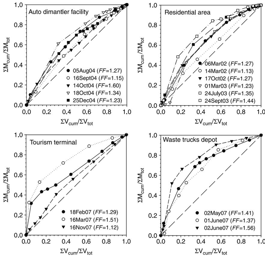
**Figure 1** M(V) curves for TSS corresponding to the mass-limited events at the auto dismantler facility, the residential site, the tourism terminal and the urban waste trucks depot. For each monitored event, the first flush index *FF* is also indicated in brackets
