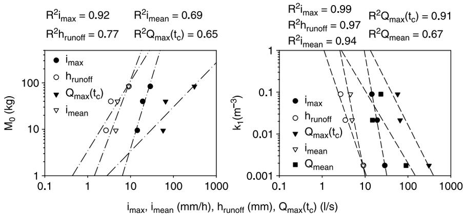
**Figure 4** Correlation between the  $M_0$  and  $k_1$  parameters and the rainfall-runoff characteristics at the tourism terminal site
