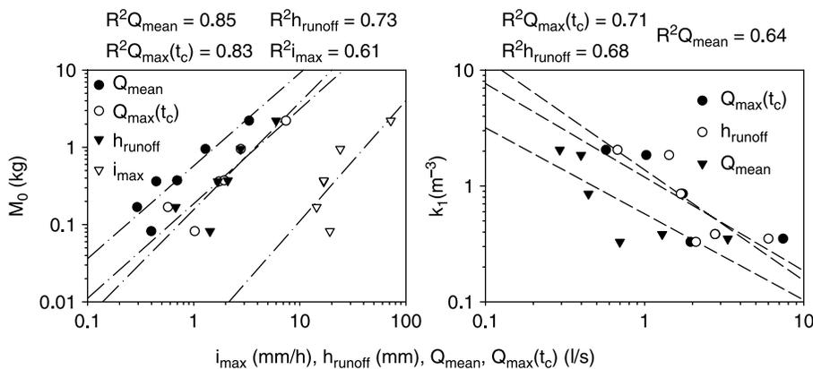
**Figure 3** Correlation between the  $M_0$  and  $k_1$  parameters and the rainfall-runoff characteristics at the residential site
