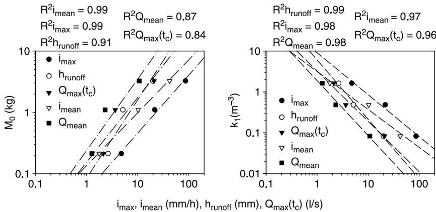
**Figure 5** Correlation between the  $M_0$  and  $k_1$  parameters and the rainfall-runoff characteristics at the urban waste trucks depot site
