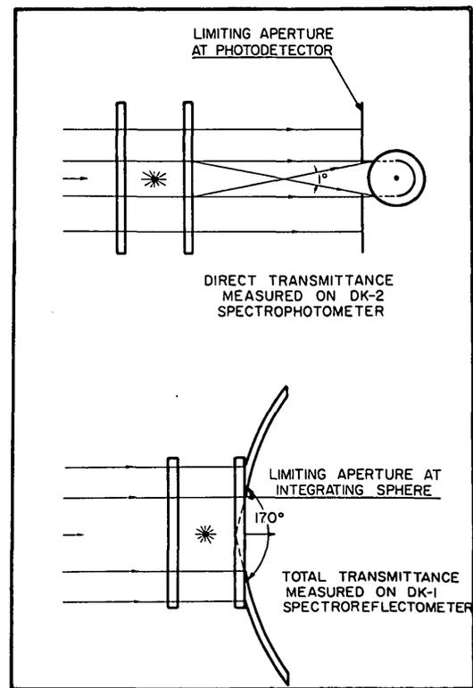
Fig. 1. Method of measuring direct and total transmittance.
