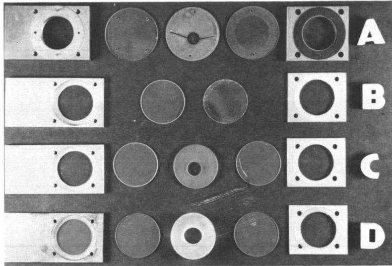
Fig. 2. Cells used to contain the ocular media.
