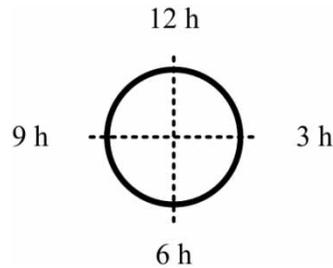
**Figure 5** | Schematic drawing of a pipe (cross-section in which the pipe positions 12 h (crown), 6 h (invert), 3 h and 9 h (springlines) are given).
