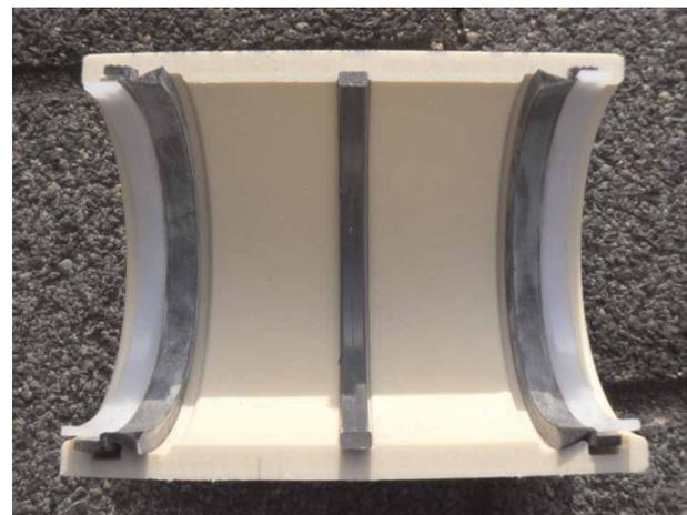
**Figure 1** | Longitudinal cut of a double-socket DN110 PVC push-fit joint. At the centre a ring (black) separates both the two pipes inside the joint. At each end a rubber gasket (black) keep the system sealed.
