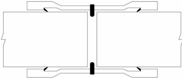
**Figure 2** | Ideal joint condition (not to scale).
