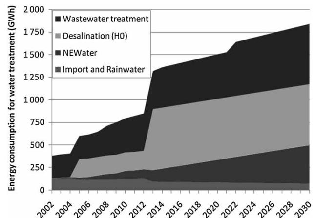
Figure 3 | Projected energy consumption for water production processes in Singapore (baseline scenario H0).
