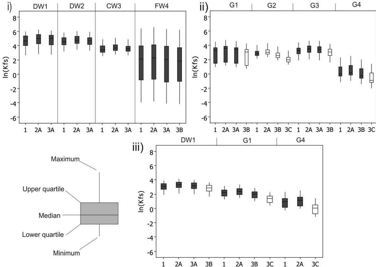
**Figure 4** | Box plots illustrating  $Kfs$  values calculated for the different sites (located in Figure 2) using solutions 1, 2A, 3A, 3B and 3C (as described in Table 2). G1, G2, G3 and G4 are grassland areas and DW1, DW2, CW3 and FW4 are woodland areas and are explained in Table 2. Open box plots have significantly different ( $P < 0.05$ ) mean  $Kfs$  values within each site group.
