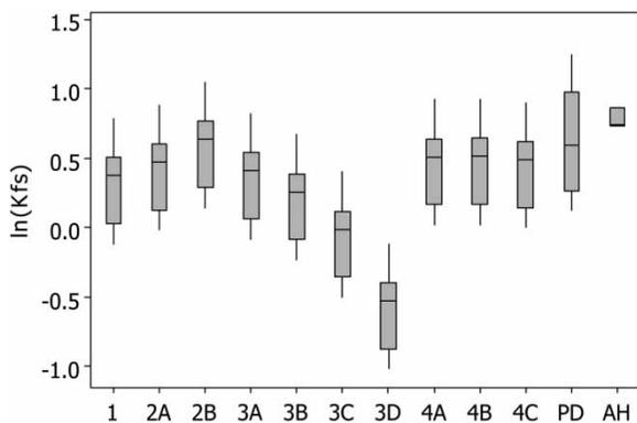
**Figure 5** | Box plot comparing log transformed  $Kfs$  results in the floodplain area (site G4) of the CHWP solutions (1, 2A, 2B, 3A, 3B, 3C, 3D, 4A, 4B, 4C), the PD and the AH methods. The description for each solution ID is given in Table 2.
