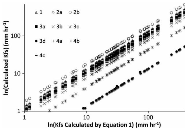
**Figure 3** | Comparison of logarithmic  $Kfs$  values calculated using different formulae described in Table 2 against the Glover solution (Equation (1)), shown as 1:1 line. The number of data points was reduced to provide more clarity to the graphs.
