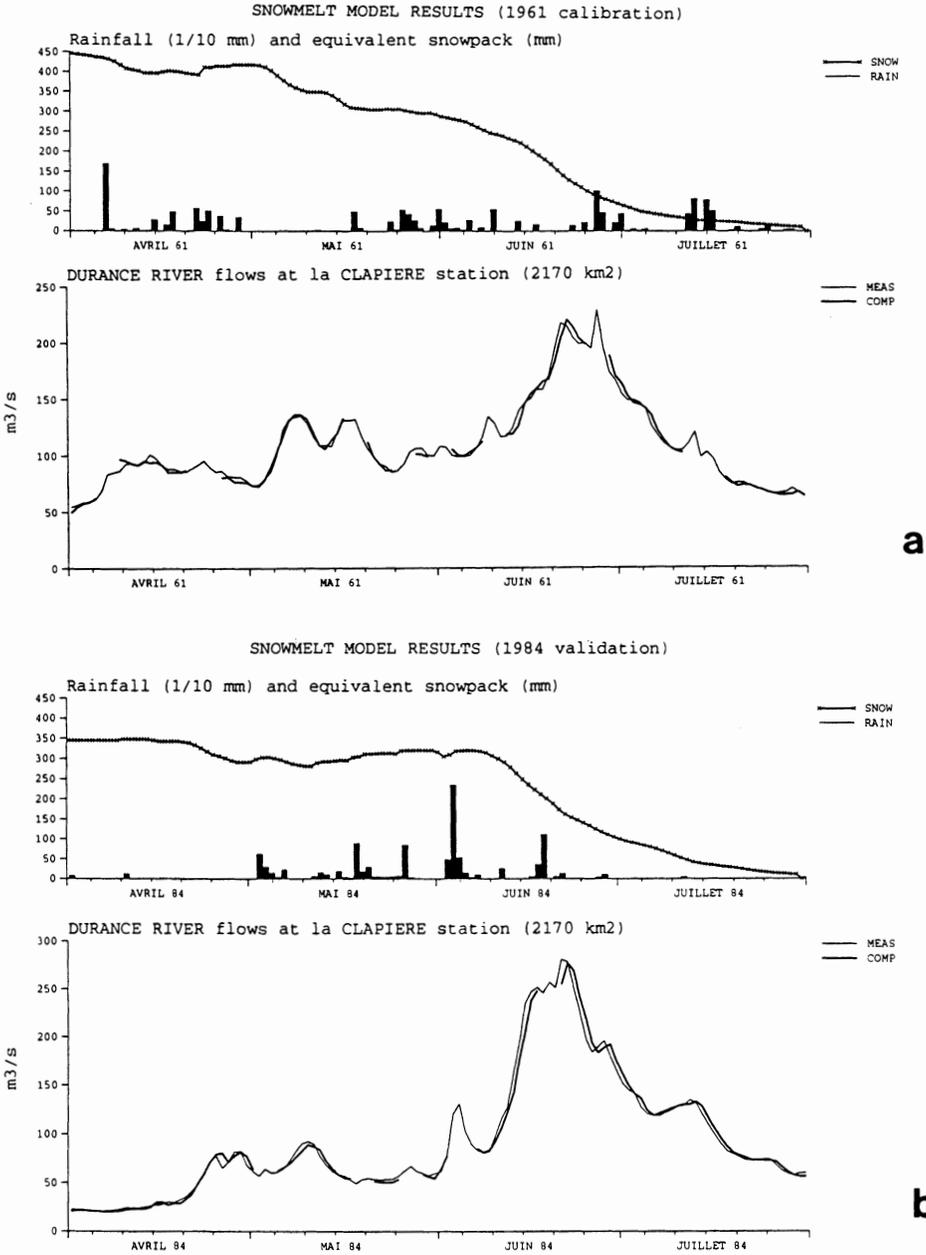
Fig. 8. Model snowmelt results (a: calibration, b: validation)
