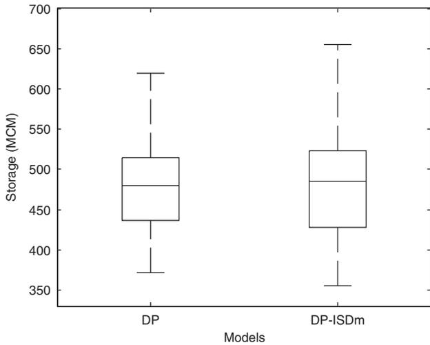
**Figure 7** | Box plot of simulated monthly storage as resulted from optimal operating rule of DP-ISDm and simple DP model.
