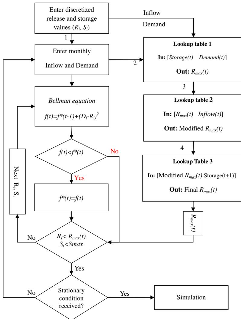
**Figure 1** | The overall structure of DP-ISD.  $R_{max}(t)$ : Maximum allowable release;  $S_{max}$ : Maximum allowable storage (reservoir capacity);  $R_i$ : Monthly release as a decision variable;  $S_i$ : Monthly storage as a state variable;  $D_i$ : Monthly demand
