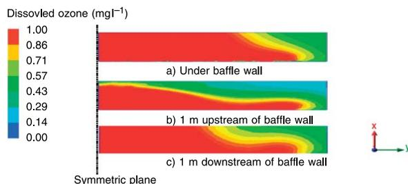
**Figure 3** | Simulated ozone residual distributions around the outlet of cell 1 in the DesBaillets WTP ozone contactor (only half of the outlet is shown).
