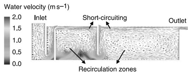
**Figure 8** | Typical velocity field in the DesBaillets WTP ozone contactor.
