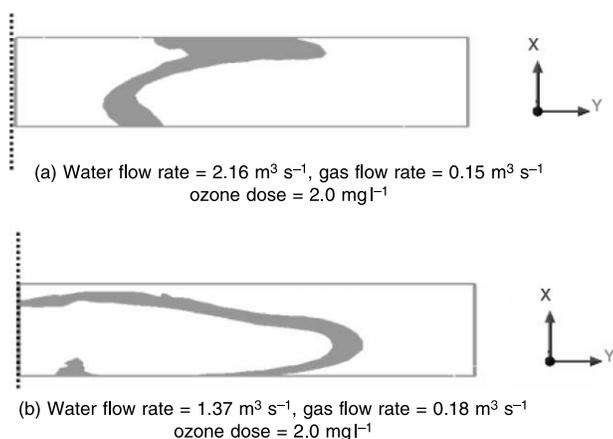
**Figure 5** | Area at the outlet of cell 1 where ozone concentrations are within  $\pm 20\%$  of the average value.
