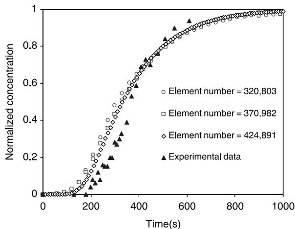
Figure 11 | Impact of the mesh density on the simulation of tracer residence time distribution.
