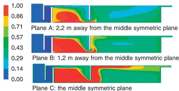
**Figure 7** | Spatial ozone residual distributions along the horizontal profile of the DesBaillets WTP ozone contactor.
