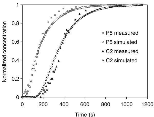
Figure 2 | Comparison of simulated and experimental tracer curves.
