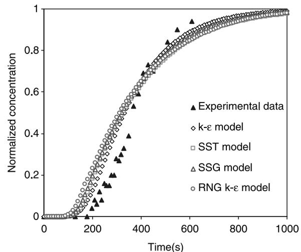
Figure 12 | Impact of the turbulence model on the simulation of tracer residence time distribution.
