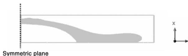
**Figure 4** | Area at the outlet of cell 1 where ozone concentrations are within  $\pm 20\%$  of the average value (water flow rate =  $3.22 \text{ m}^3 \text{ s}^{-1}$ ; gas flow rate =  $0.21 \text{ m}^3 \text{ s}^{-1}$ ; ozone dose =  $2.2 \text{ mg l}^{-1}$ ).
