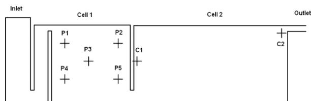
**Figure 1** | Ozone residual sampling ports in a DesBaillets WTP ozone contactor.
