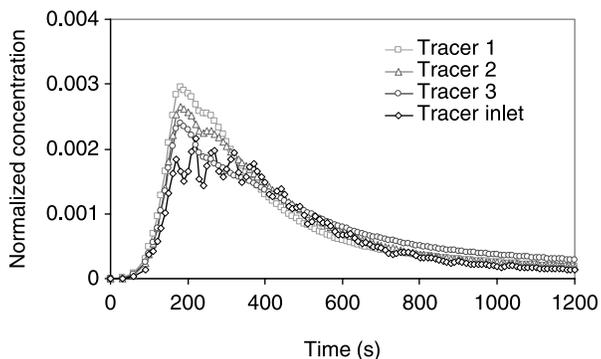
**Figure 9** | Effects of tracer injection location on tracer residence time distribution.
