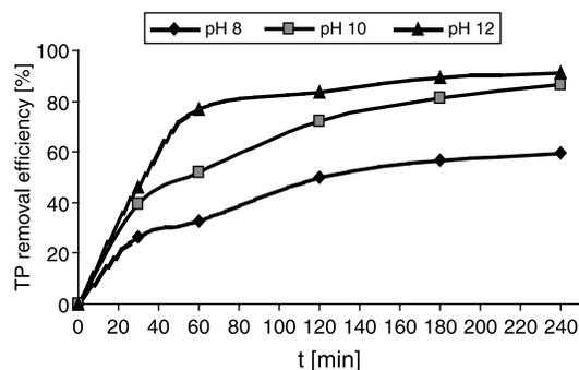
**Figure 1** TP removal trends during ozonation tests carried out at initial pH values of 8, 10 and 12
