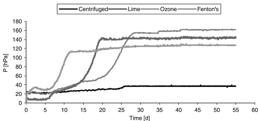
**Figure 6** Pressure trends during anaerobic tests**Table 8** Anaerobic tests
