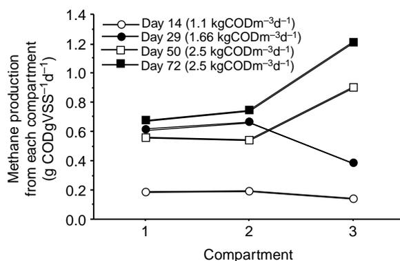
Figure 1 Profiles of methane production during progress through the baffled reactor
