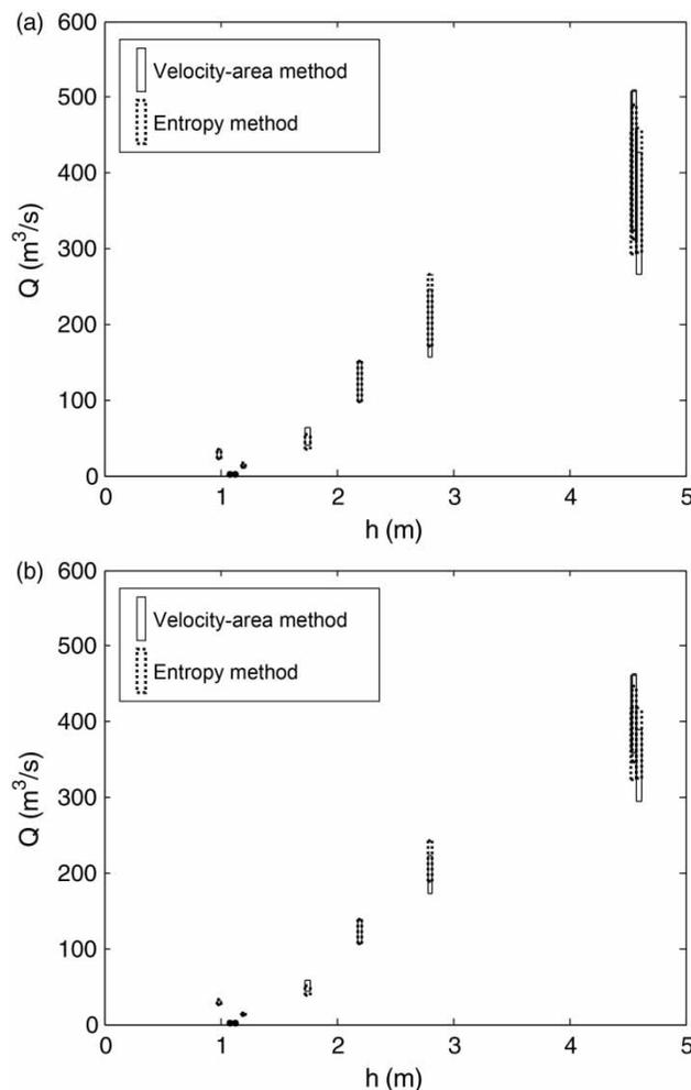
**Figure 9** | Equipped section – Ponte Felcino: comparison between the grey discharges estimated through the velocity-area method greyified (a) through the type I approach and (b) through the type II approach, with the corresponding grey discharges estimated through the grey entropy method.
