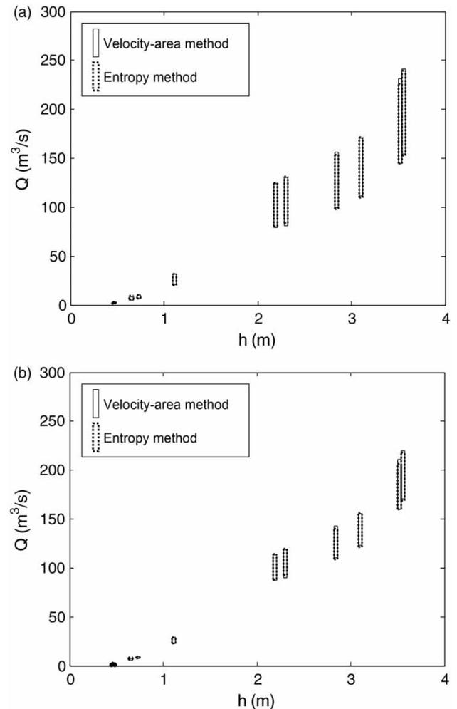
**Figure 10** | Equipped section – Santa Lucia: comparison between the grey discharges estimated through the velocity-area method greyified (a) through the type I approach and (b) through the type II approach, with the corresponding grey discharges estimated through the grey entropy method.
