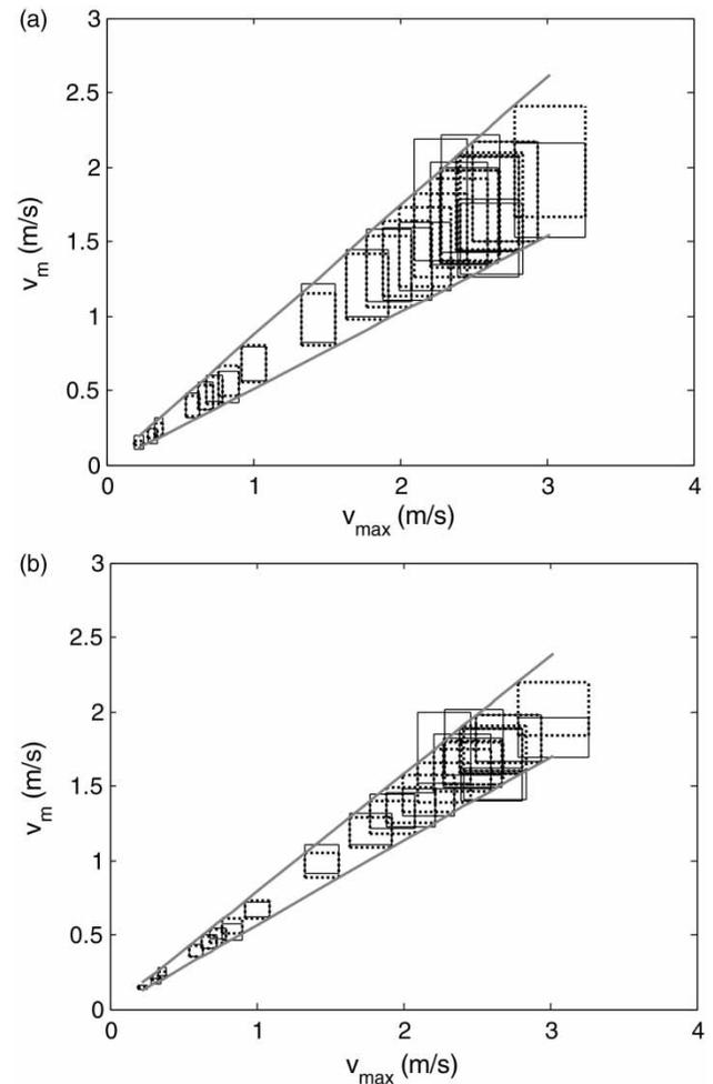
**Figure 7** | Equipped section – Ponte Nuovo: greyified entropy method. Comparison between the mean velocities obtained through the velocity-area method greyified (a) through the type I approach and (b) through the type II approach (black solid line) with those estimated on the basis of the grey maximum velocity given by Equation (20) (black dashed line).
