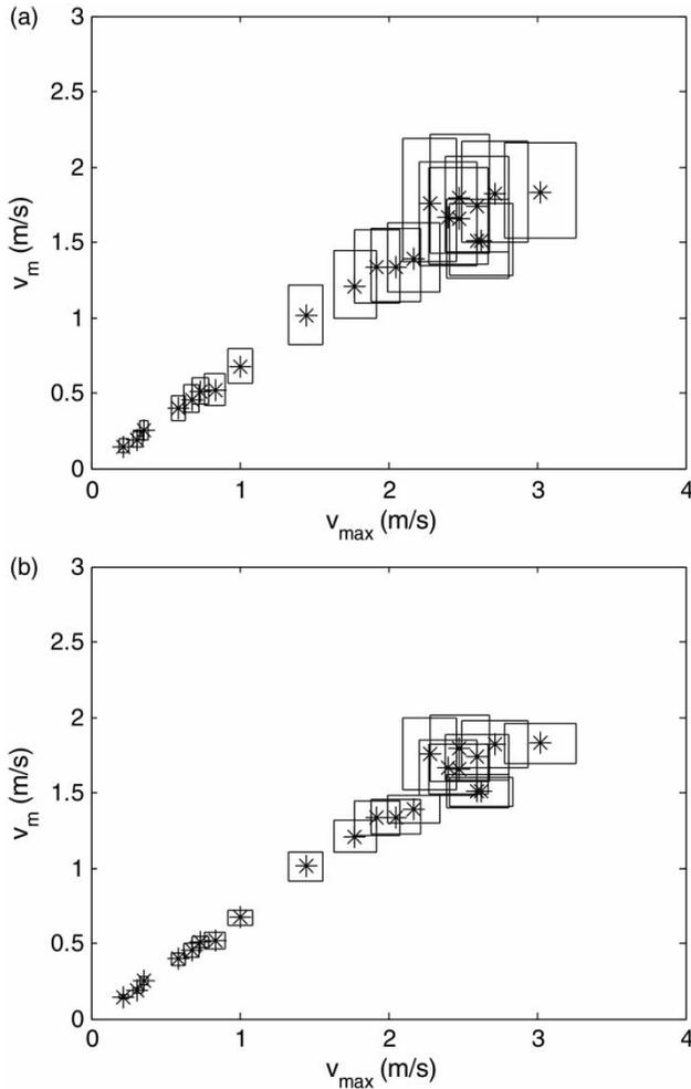
**Figure 6** | Equipped section – Ponte Nuovo: grey quantification of the uncertainty on the maximum and mean velocities. The uncertainty pertaining to the mean velocities is obtained through the use of the velocity-area method greyified (a) through the type I approach and (b) through the type II approach.
