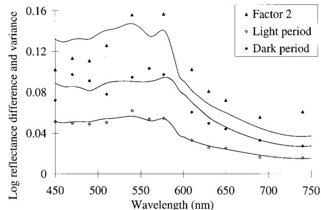
FIGURE 7. Slow reflectance changes expressed as log reflectance difference and variance with model fits.<sup>22</sup> Filled triangles indicate data gathered from the factor analysis described in Figure 3. Filled and empty diamonds indicate data log reflectance changes between 6 and 34 minutes in the dark and between 2 and 15 minutes in the light, respectively. Fits for the latter two were better than for the factor analysis.
