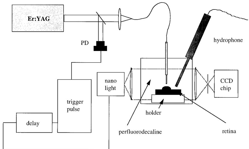
**FIGURE 3.** Schematic drawing of the fast flash shadow imaging. The flash light is controlled by the Er:YAG laser via a trigger/delay unit. A CCD chip records the shadow image. A needle hydrophone was used to measure laser-induced pressure transients at a distance of 2 mm to the fiber tip.
