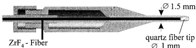
FIGURE 1. Schematic picture of the laser radiation delivery handpiece.
