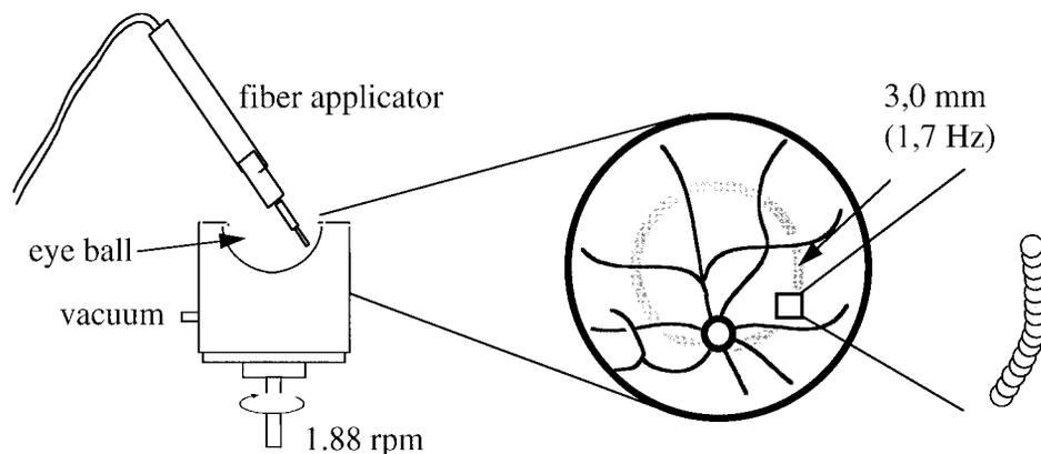
FIGURE 2. Laser experiments: Schematic drawing showing the experimental setup and the pattern of laser application. The laser energy was delivered on a circular path with a 3-mm radius. The individual laser spots were applied in such a way that a 50% overlap of the individual spots was achieved.
