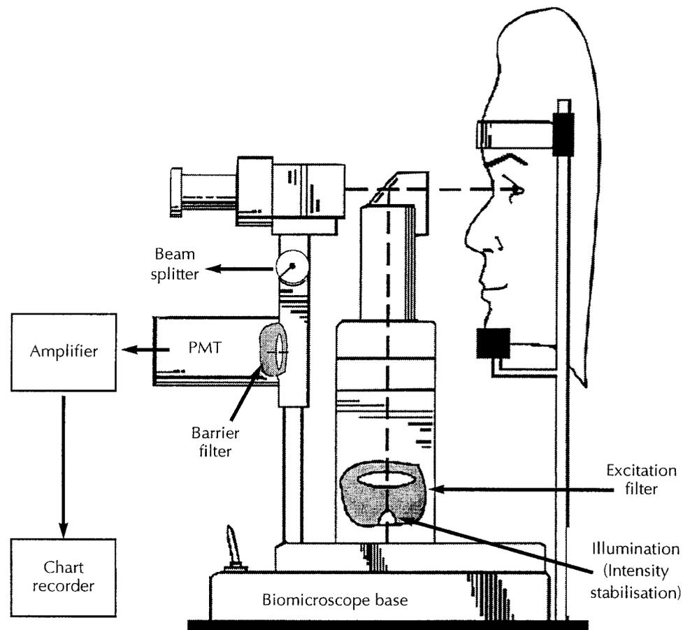
**FIGURE 1.** Schematic diagram of the biomicroscope fluorometer. The base instrument incorporated a beam splitter for rapid switching from viewing to recording through a side-on photomultiplier. The illumination was stabilized with a voltage-feedback system.
