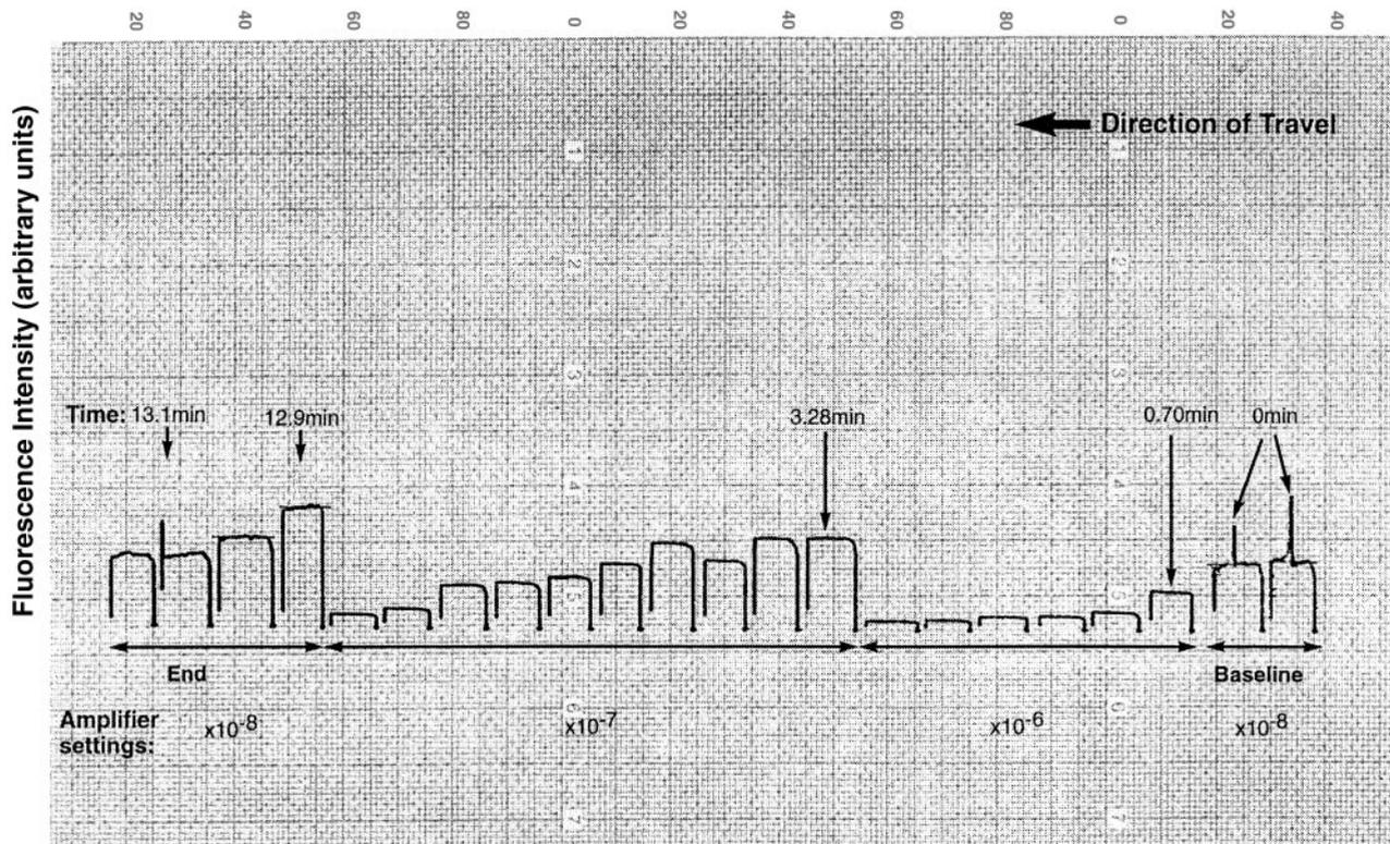
FIGURE 2. Sample chart recorder trace. Square waves represent recording periods of 2 to 4 seconds.
