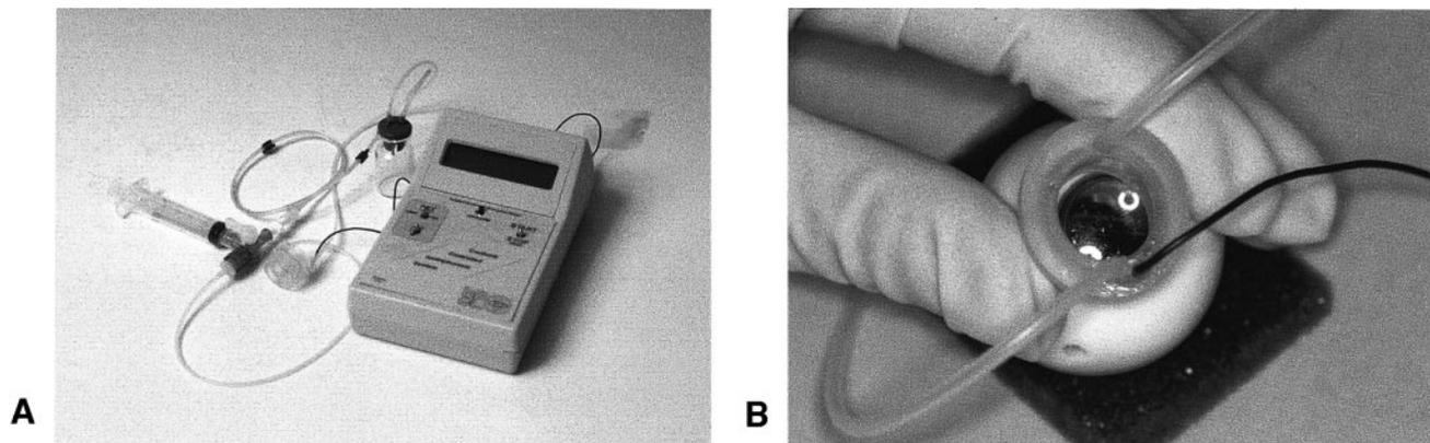
**FIGURE 1.** CCI system. (A) Battery-operated programmable control unit connected to the ocular applicator with fluidic lines connected to a syringe and the drug reservoir. (B) Autoclavable silicone rubber CCI ocular applicator shown on a plastic model eye.
