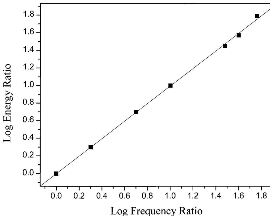
FIGURE 5. A comparison of the log frequency values of the pulses driving the LEDs with the measured log ratio energy output produced by these changes in frequency.
