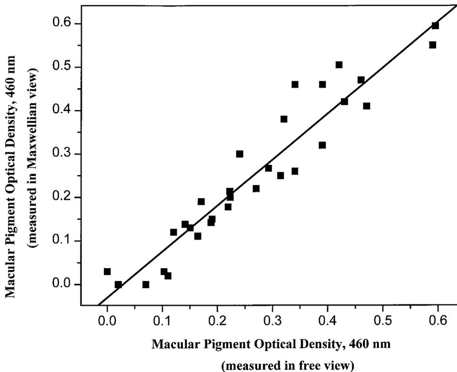
FIGURE 6. The relationship between MP optical density measured in Maxwellian view and MP density measured with the tabletop LED device in free view.
