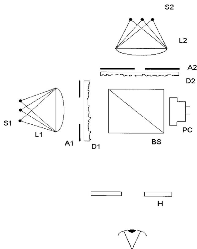
FIGURE 3. A schematic of the optical system used to measure MP optical density in free view. A1 and A2, Apertures 1 and 2; BS, beam splitter; L1 and L2, planoconvex achromatic lenses; PC, photocell; H, hot mirror used to reduce heat transmission; S1 and S2, light sources; D1 and D2, optical diffusers.
