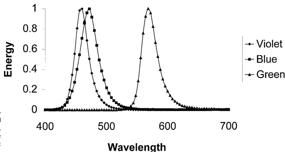
FIGURE 4. The relative spectral energy curve of the LEDs that were used to create the background (*squares*), measuring (*diamonds*), and reference (*triangles*) fields for the measurement of MP with the tabletop device.
