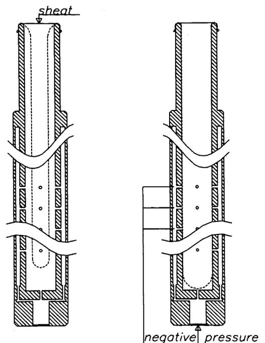
**Fig. 1.** Inner and outer Perspex or Polycarbonate tubes. Negative pressure is applied to the space between the inner and outer tubes. The suction force is transferred to the inner tubes via holes in the inner tube and at the bottom. The inner tube is sealed airtight to the outer tube.
