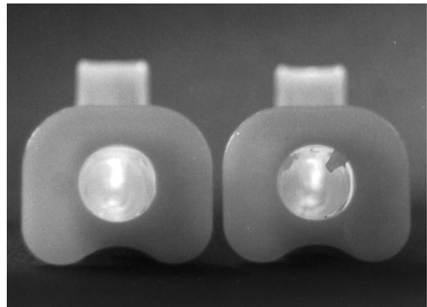
**Fig. 1.** Side-by-side comparison of a normal Williams intubating airway (*left*) and the faulty one (*right*). Note a protruding plastic piece (“tooth”) in the circular lumen of the faulty airway, at approximately the 2 o'clock position. A second “tooth” was located at the 10 o'clock position and has been dislodged after passing an endotracheal tube.
