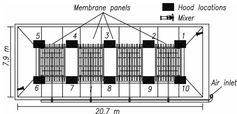
Figure 2 | Diagram of the test tank indicating the sampling locations (from 1 to 10) and diffuser mixer positions.
