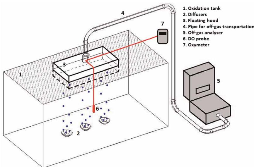
Figure 1 | Functional off-gas test diagram.
