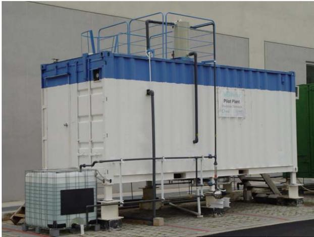
**Figure 2** | Containerized pilot RO plant.
