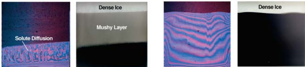
Hypo-eutectic Aqueous Solution, C_i=5\text{wt}\%
