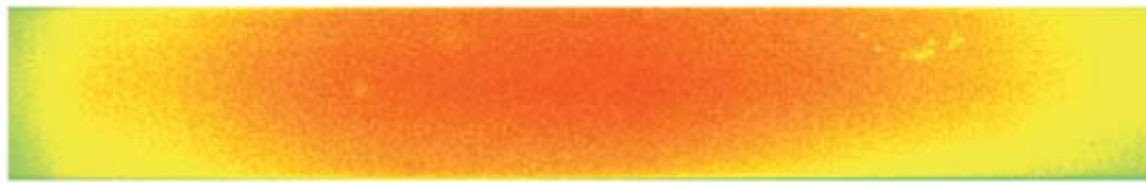
(c) Raw image of temperature-dependent rhodamine B fluorescence intensity at \lambda = 580 \text{ nm}
