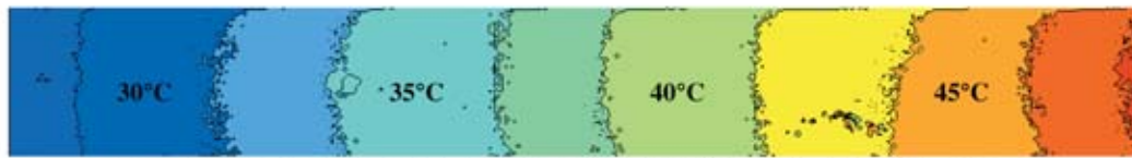
(d) Contour plot of processed temperature field showing 2.5°C isotherms
