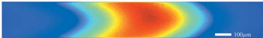
(e) Focusing of bodipy sample in thermal gradient shown in (d) with E = 40 \text{ V/mm} and \lambda = 530 \text{ nm}
