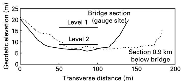
**Figure 2** River cross-sections in the vicinity of the gauging station. Level 1 = highest ice-influenced stage on record (1970); level 2 = stage on date of survey, 12 July 1999; a typical winter stage is about 0.8 m higher than the level 2
