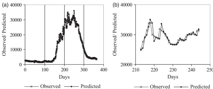
**Figure 4** | Observed and predicted series values (in m<sup>3</sup>/s) for validation data using model Equation (17). (a) for the whole year 1994; (b) only August is focused on for better clarity.
