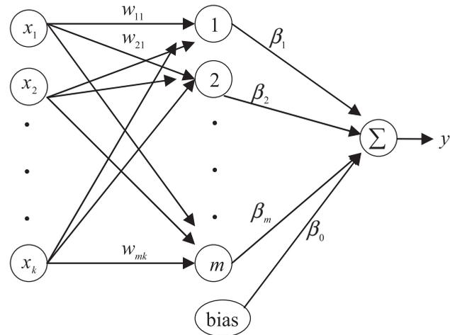
Figure 1 | Architecture of product units based neural network.
