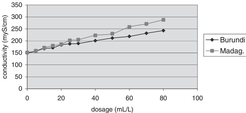
**Figure 2** Conductivity measurements of non-shelled seeds from Burundi and Madagascar (RM: 2 min. at 160 rpm; SM: 20 min. at 40 rpm; ST: 30 min.)
