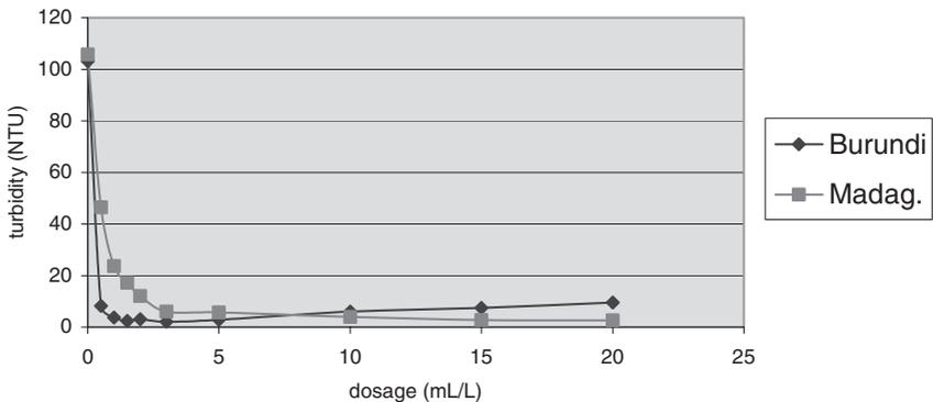
**Figure 3** Turbidity measurements of shelled seeds from Burundi and Madagascar (RM: 2 min. at 100 rpm; SM: 20 min. at 40 rpm; ST: 30 min.)
