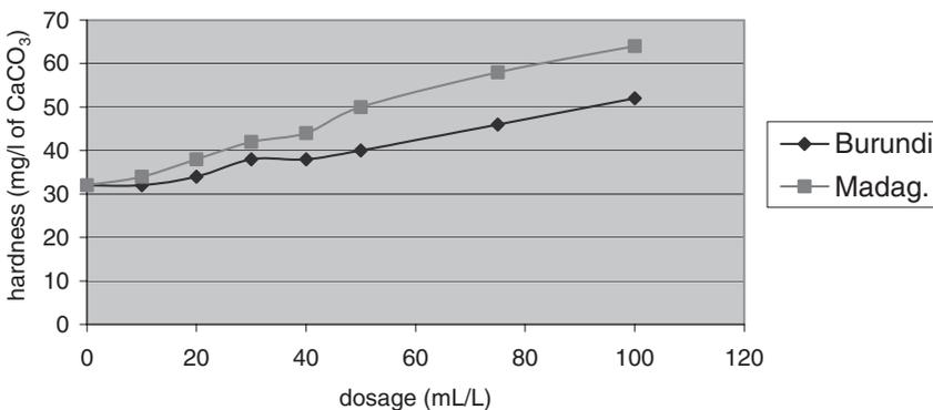
**Figure 5** Hardness measurements for seeds from Burundi and Madagascar (RM: 2 min. at 100 rpm; SM: 20 min. at 40 rpm; ST: 30 min.)
