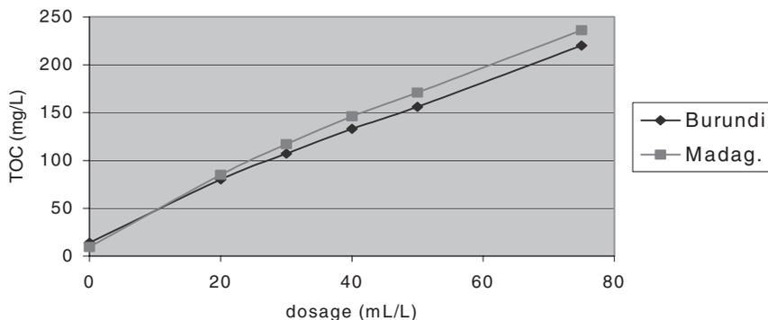
**Figure 6** Total organic carbon measurements on seeds from Burundi and Madagascar (RM: 2 min. at 100 rpm; SM: 20 min. at 40 rpm; ST: 30 min.)
