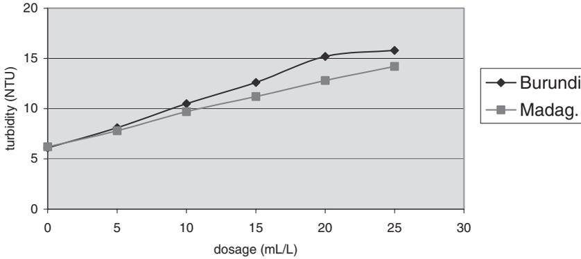
**Figure 4** Turbidity measurements for non-shelled seeds for the removal of low turbidity of 6 NTU (RM: 10 s at 160 rpm; SM: 5 min. at 30 rpm; ST: 20 min.)
