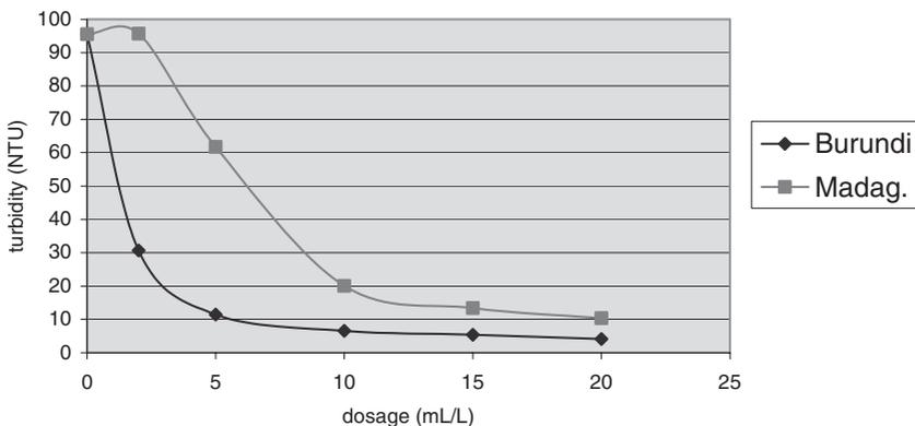
**Figure 1** Turbidity measurements for non-shelled seeds from Burundi and Madagascar (RM: 2 min. at 160 rpm; SM: 20 min. at 40 rpm; ST: 30 min.)
