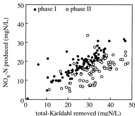
**Figure 3** Relationship between the removal of total (unfiltered) Kjeldahl-nitrogen and the formation of oxidized-form nitrogen in the DHS unit during phase I and phase II
