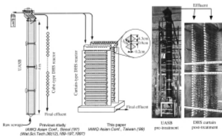
**Figure 1** Schematic diagram and photograph of an experimental setup (USAB unit plus certain-type DHS unit) installed at a sewage treatment site. For reference the cube-type DHS process used in the previous study is also presented in the figure
