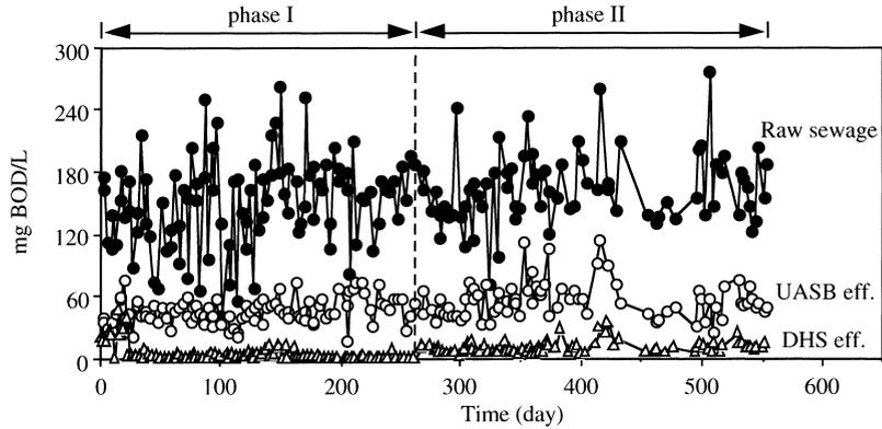
**Figure 2** Time course of total-BOD of raw sewage, of UASB effluent, and of curtain-type DHS effluent during the phase I and the phase II experiments
