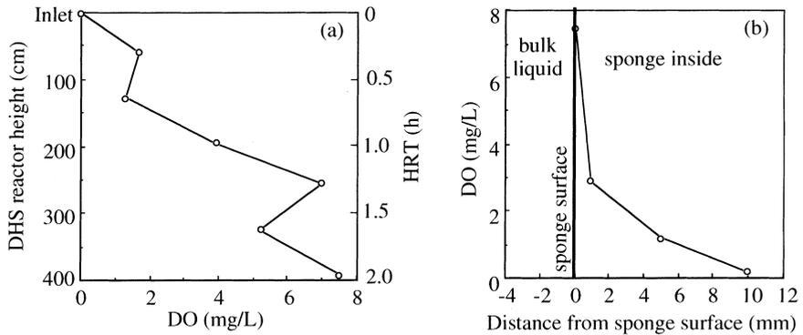
**Figure 5** Profiles of dissolved oxygen in the curtain-type DHS determined by using a DO microelectrode. (a) along the reactor height; (b) sponge-inward depth
