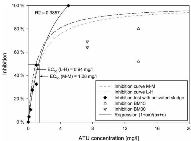
**Figure 4** | Inhibition curves of ATU and adaption results of BM15 and BM30.
