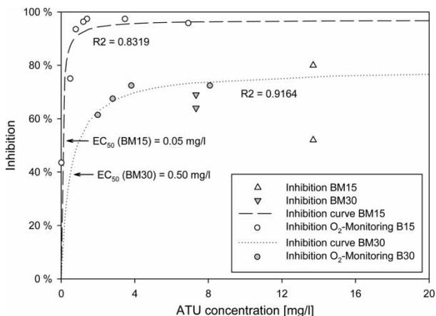
Figure 7 | ATU-inhibition curves of BM15 and BM30.
