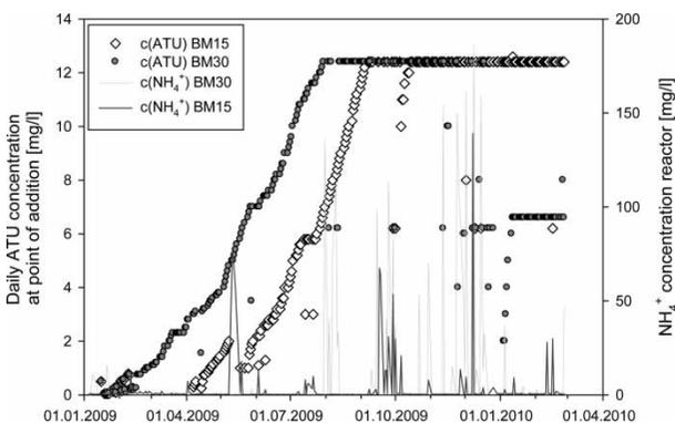
**Figure 3** | Stepwise increase of ATU concentration for BM15 and BM30 and their respective ammonia concentration at the end of the day and before the next NH<sub>4</sub><sup>+</sup> addition.
