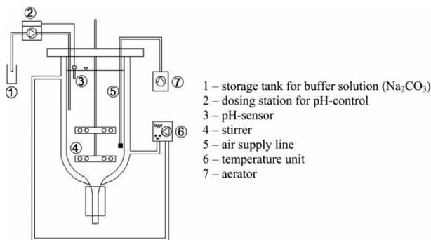
Figure 2 | Reactor configuration.
