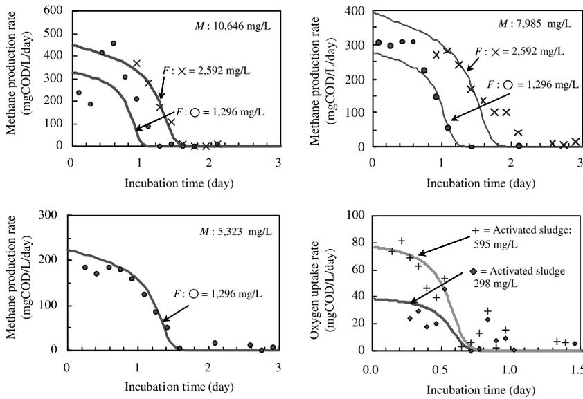
**Figure 6** Respirograms for the degradation of  $X_{S2}$  and  $X_S$  under various F/M ratio conditions, upper left, lower left and upper right: anaerobic respirogram for  $X_{S2}$ , comparison based on type II; lower right: aerobic respirograms for  $X_S$  (activated sludge only)
