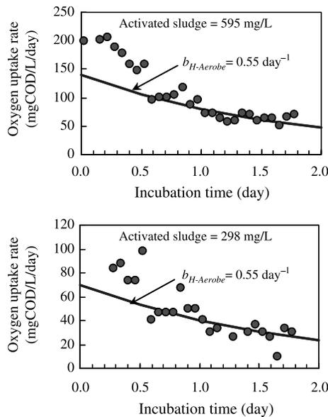
**Figure 5** Decay of  $X_{H-Aerobe}$  in the aerobic condition
