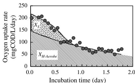
**Figure 3** Respirogram in aerobic condition, activated sludge: 595 mg/L
