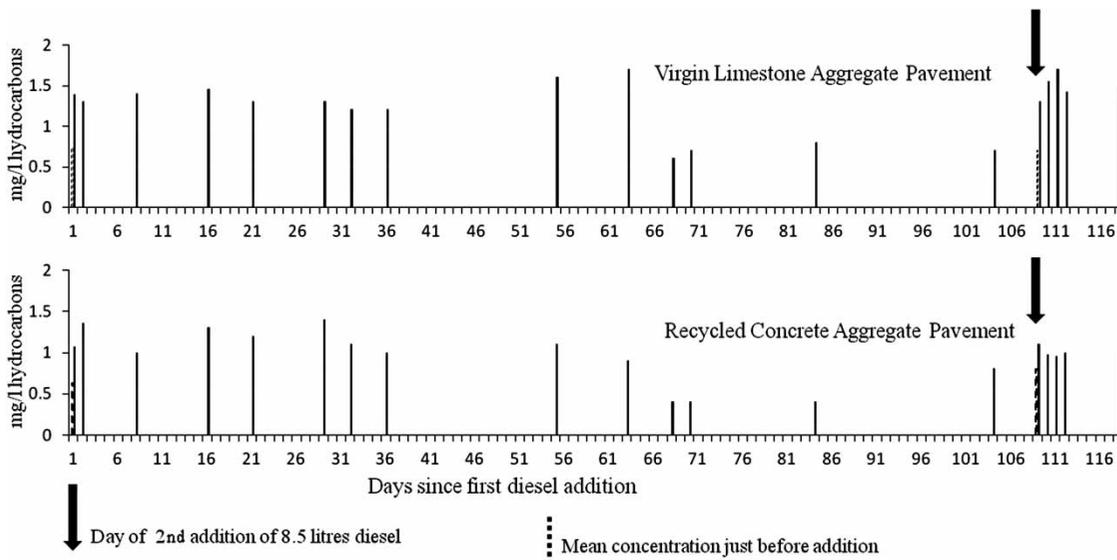
**Figure 5** | Mean daily oil concentration on days from first diesel addition (days D1–D119).
