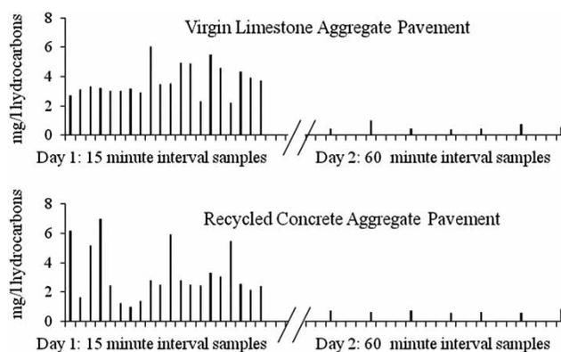
**Figure 3** | Hydrocarbon concentrations in effluent. First 2 days after lubricating oil addition (nominal time series over 28 hours days L1 and L2).
