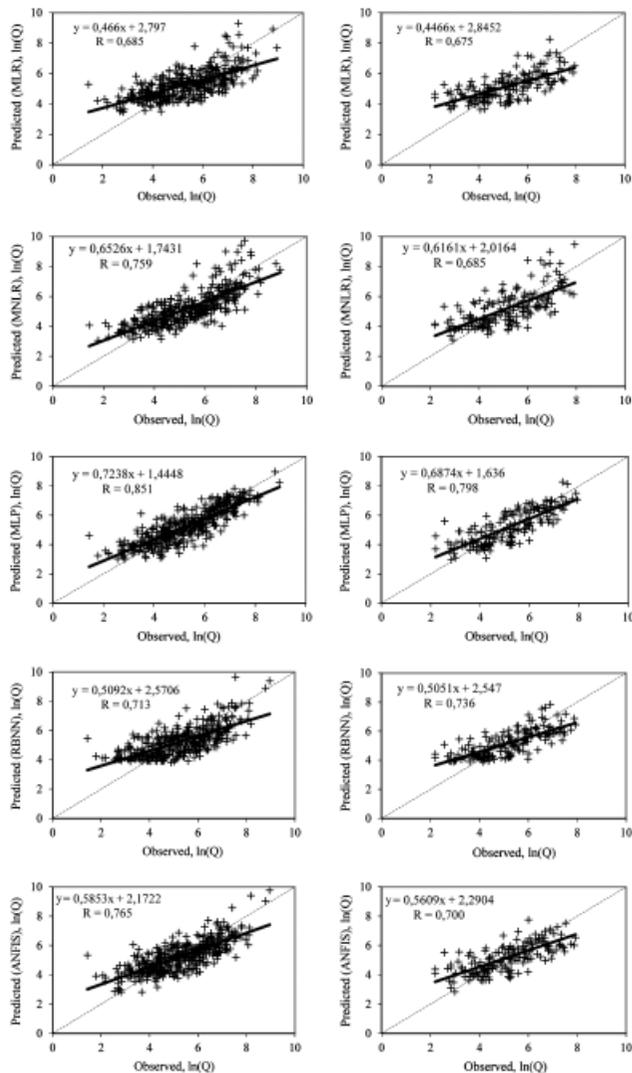
**Figure 2** | Comparison of the observed and predicted maximum discharge values using MLR, MNLR, MLP, RBNN and ANFIS models during training (left column) and testing (right column) phases.
