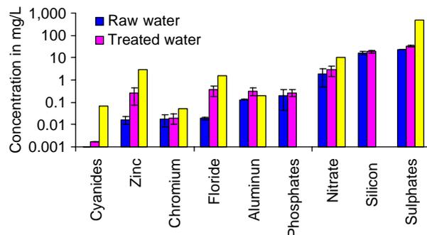
Figure 5 | Historical data of raw and treated water parameters regularly monitored at Kadahokwa WTP for the period July to October 2007 (mean  $\pm$  StDev,  $n = 5$ ), and related WHO toxicity limits (House & Reed 2004; LENNTECH 2006).
