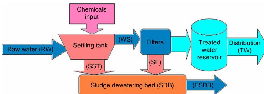
Figure 3 | Sampling sites at Kadahokwa water treatment plant.
