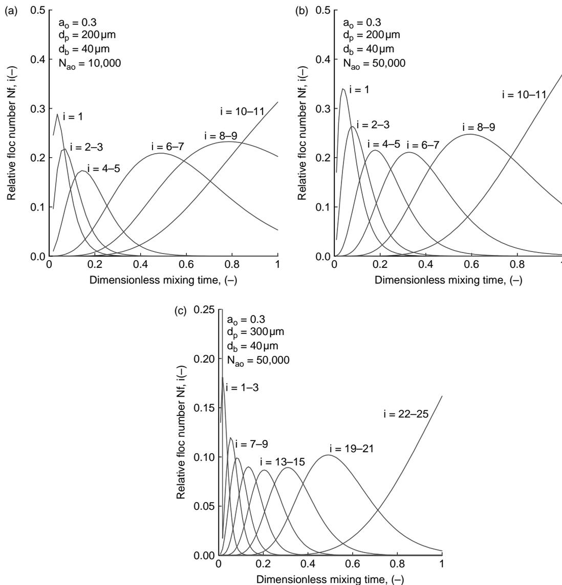
Figure 2 | Number of attached bubbles on a floc simulated in terms of mixing (contact) time.
