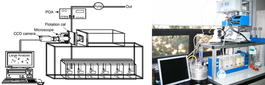
Figure 1 | Schematic diagram and photograph of the jar tester equipped with bubble-supplying apparatus and PIA.
