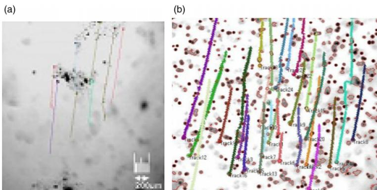
**Figure 4** | Photograph of rise velocity tracking: (a) captured image from CCD camera; (b) tracking image of bubble-floc agglomerates.
