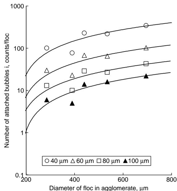
**Figure 6** | Calculated number of attached bubbles on a floc as a function of bubble diameter.
