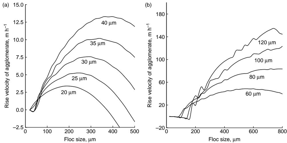
**Figure 3** | Maximum rise velocity of bubble/floc agglomerates as a function of bubble diameter.
