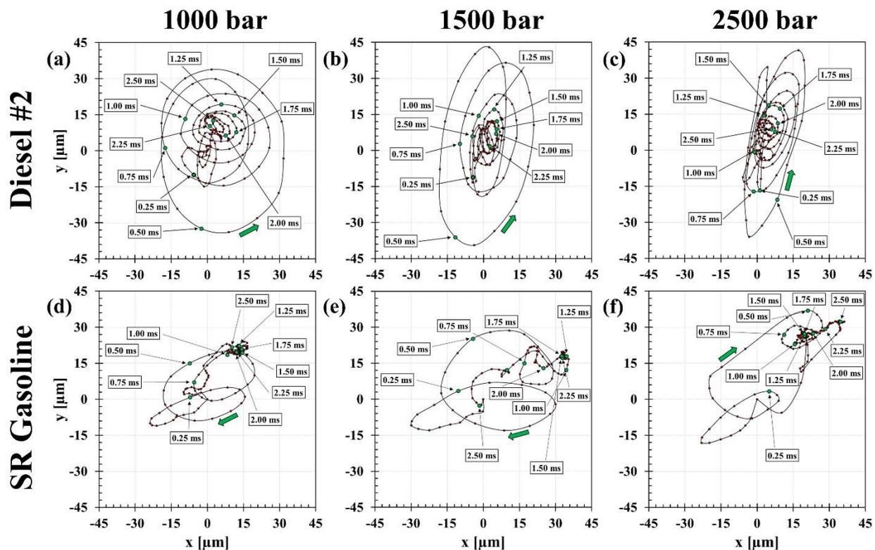
Figure 1. Average lateral motion path of the injector needle at 1000 (a, d), 1500 (b, e) and 2500 bar (c, f) injection pressures for diesel #2 (a, b, c) and SRG (d, e, f) fuels respectively. a), b), and c) are taken from [9].
