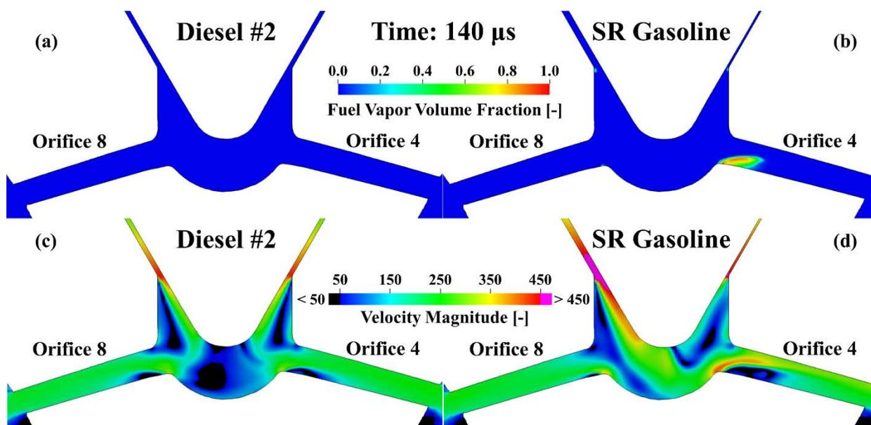
Figure 3. Contours of fuel vapor volume fraction (a, b) and velocity magnitude (c, d) at 140  $\mu$ s using diesel #2 (a, c) and SRG (b, d) fuels respectively. The results are plotted on a plane that crosses through orifice 4 and 8 and includes the injector symmetry axis.
