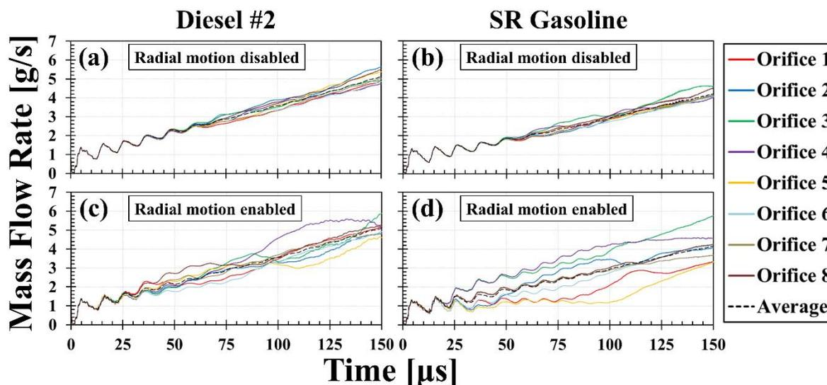
Figure 2. Orifice mass flow rates at 1000 bar injection pressure with radial motion disabled (a, b), and enabled (c, d) using diesel #2 (a, b) and SRG (c, d) fuels respectively. The results plotted in (a) and (c) are extracted from [9].
