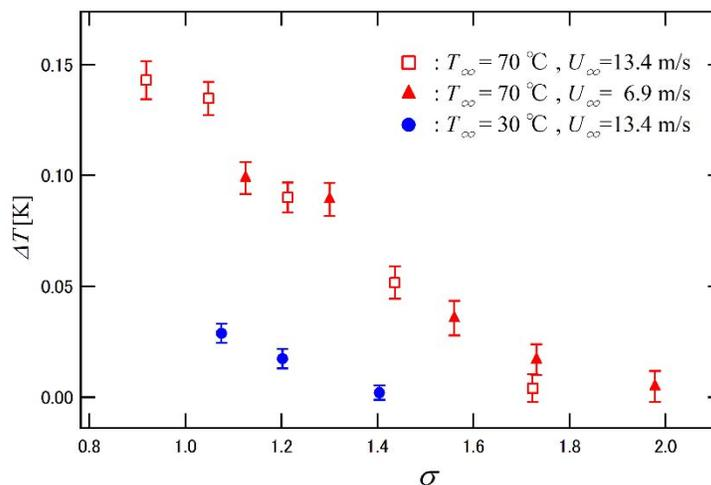
Fig.3 Temperature depression inside a cavity at angle of attack  $\alpha = 9\text{ deg}$ .
