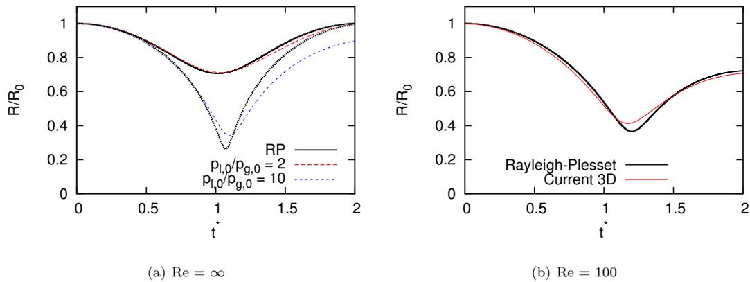
Figure 2: Bubble radius evolution for two different collapse intensities,  $p_{l,0}/p_{g,0} = 2$  and  $p_{l,0}/p_{g,0} = 10$ . Color lines represent the solution obtained with current 3D simulations, black lines represent the solution obtained with a Rayleigh Plesset model.
