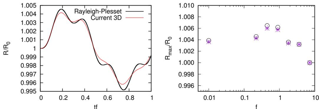
Figure 1: Left: Temporal evolution of the averaged bubble radius compared with the Rayleigh-Plesset model for the low frequency limit case  $\frac{\omega}{\omega_N} = 0.25$ . Right: Amplitude of the bubble oscillation as a function of the excitation frequency with the current method and the Rayleigh-Plesset model.
