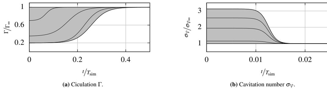
**Figure 1:** Ranges and evolution of the circulation  $\Gamma$  and cavitation number  $\sigma_V$  over time  $t$  with respect to the duration of the simulation  $T_{sim}$ .  $\Gamma_\infty$  and  $\sigma_{V\infty}$  denote the final circulation and cavitation number, respectively. While the thick lines show the limits for possible slopes, the thin lines hint randomly varying slopes.
