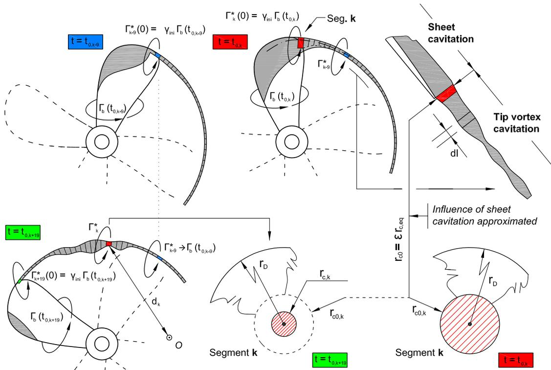
**Figure 4:** Segmentation scheme of the propeller tip vortex cavitation model. Also showing the influence of sheet cavitation on the dynamic behaviour of tip vortex cavitation.
