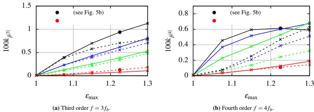
**Figure 6:** Influence of the viscous core radius  $r_{a0}$  and the exaggeration factor  $\varepsilon_{\max}$  for the full-scale configuration (solid lines) and the model configuration (dashed lines). Colour code:  $2 \cdot 100 r_{a0}/D = \{ \bullet 1.067, \bullet 1.333, \bullet 1.6, \bullet 1.867 \}$ . The filled circles correspond to the exemplary cases in Figure 5b.
