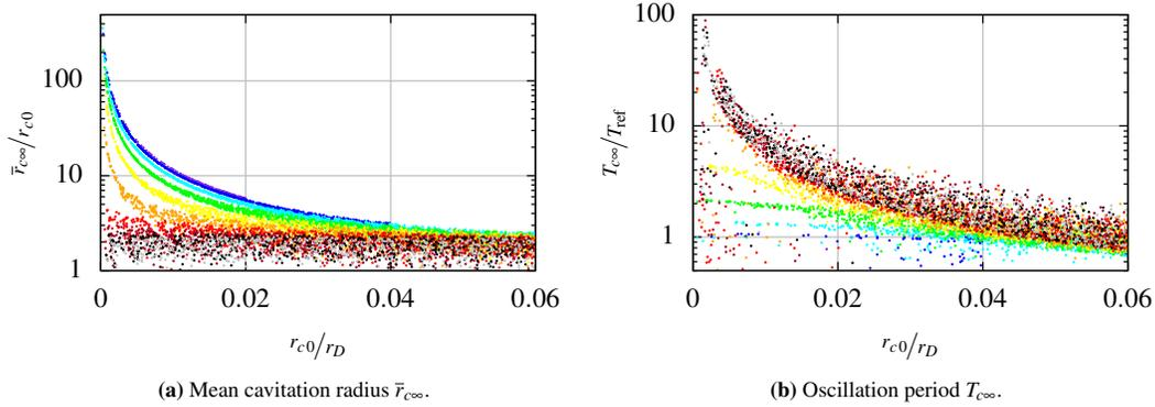
**Figure 3:** Exemplary simulation results with respect to oscillation period  $T_{c\infty}$  and mean cavitation radius  $\bar{r}_{c\infty}$  at the end of the simulation. Each dot indicates one simulation result. Colour code:  $r_{a0}/r_D = \{0.02, 0.04, 0.06, 0.08, 0.1, 0.12, 0.14, 0.16, 0.18, 0.2\}$ .
