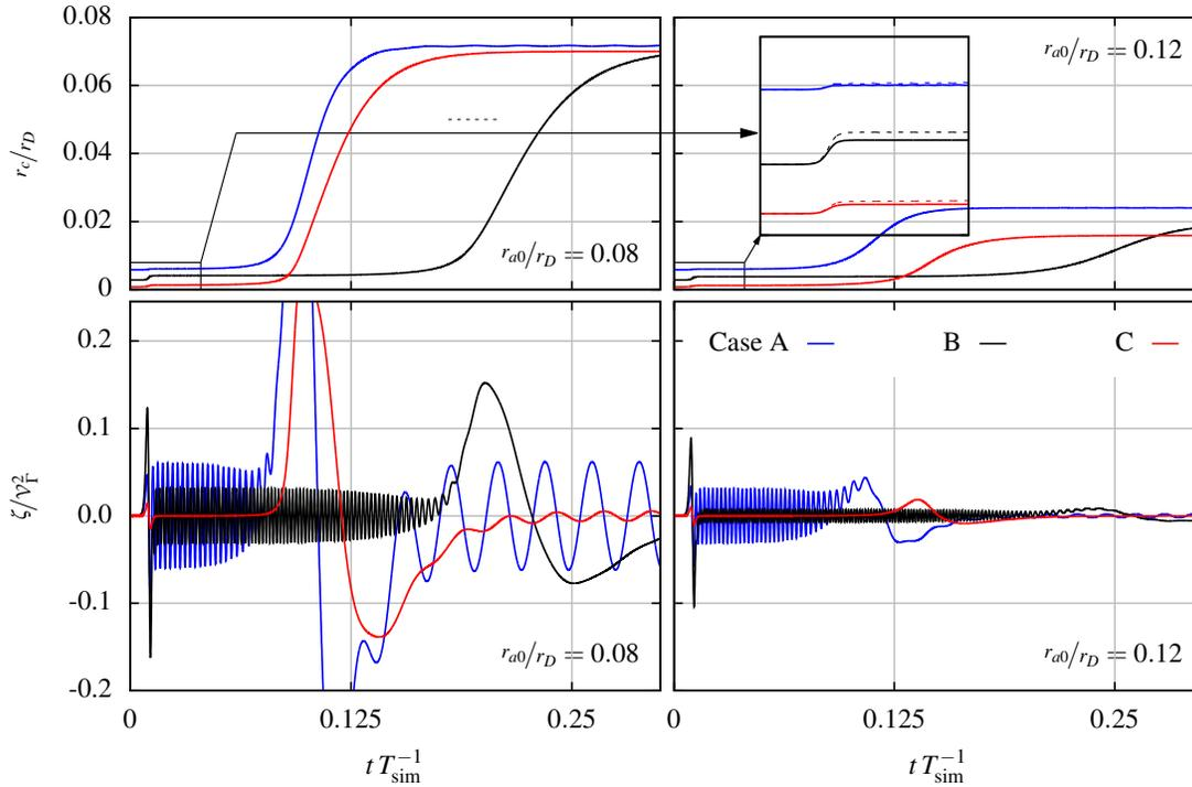
**Figure 2:** Three exemplary bubble evolutions for the cases listed in the table below for  $r_{a0}/r_D = 0.08$  (left) and  $r_{a0}/r_D = 0.12$  (right) resembling full-scale and model conditions, respectively. Top: evolution of the cavity radius  $r_c(t)$ ; bottom: pseudo radiated pressure  $\zeta$  (see text for definition).
