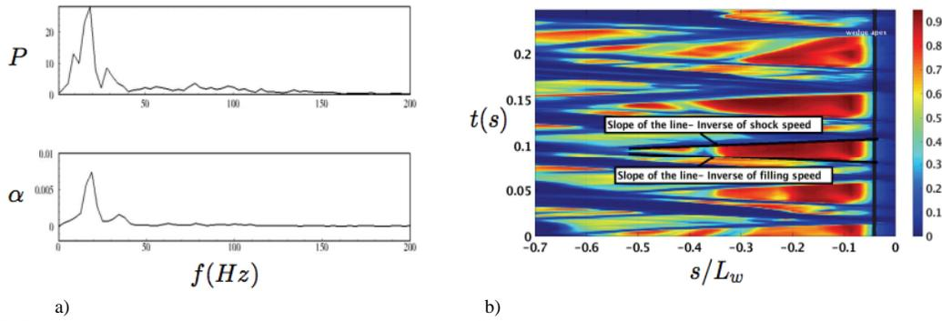
Figure 6. a) PSD of pressure and volume fraction taken inside cavity at 1.5h downstream of wedge apex. b) Contours of vapor volume fraction taken parallel to the surface of wedge for 0.25s (roughly 4-5 shedding cycles)
