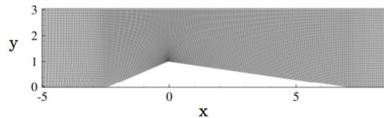
Figure 2. 2D-slice of the computational mesh close to the wedge (dimensions are in inches)
