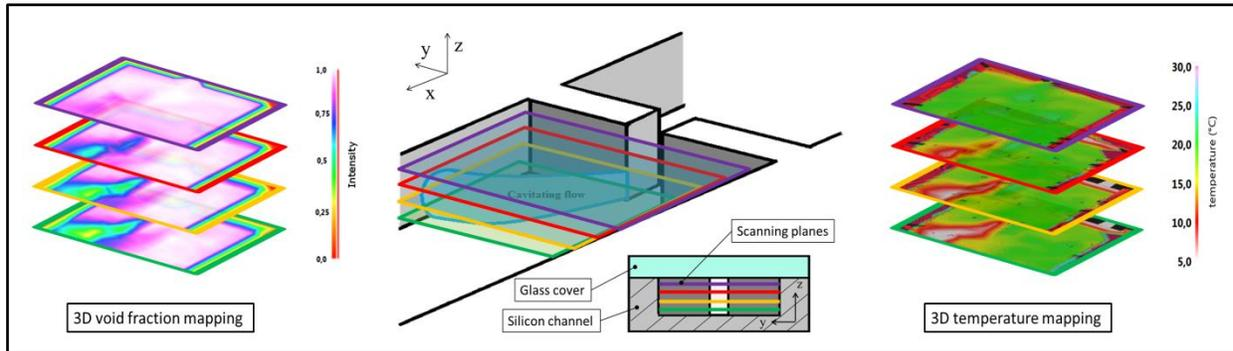
Figure 2: Raster scanning 2d planes at different heights makes 3d characterization of the channels possible. The recorded planes are recorded 20, 50, 70 and 90µm from the transparent wall (cover glass) of the microchannel. The observed two-phase flow and the associated cooling is predominantly located towards the silicon channel wall
