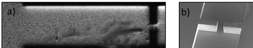
Figure 1: a) Example of cavitating flow in microfluidic channel (8bar driving pressure); flow from right to left. b) SEM image of etched silicon, before sealing the channel with a Pyrex cap. Opening of the constriction in both cases is about 80µm.
