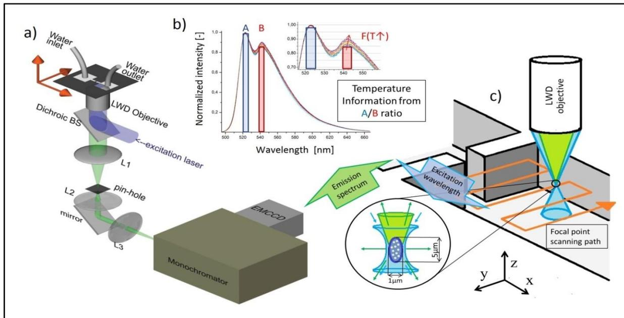
Figure 3: a) confocal microscope detection system, b) emission spectra varying with temperature, ratio of the two peaks yields a value corresponding to a certain temperature, c) focal point raster scanning and emission voxel with excited fluorophores in the nanoprobe producing the emission spectrum.
