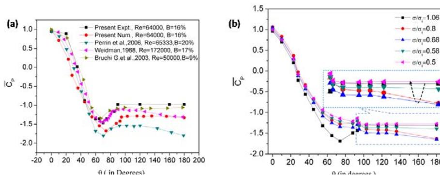
Figure 2: (a) Non-cavitating mean pressure coefficient ( $C_p$ ) for  $\sigma/\sigma_i = 1.06$  (b) Mean pressure is plotted for different cavitation numbers. Present Expt. is referred to experiments conducted [19].
