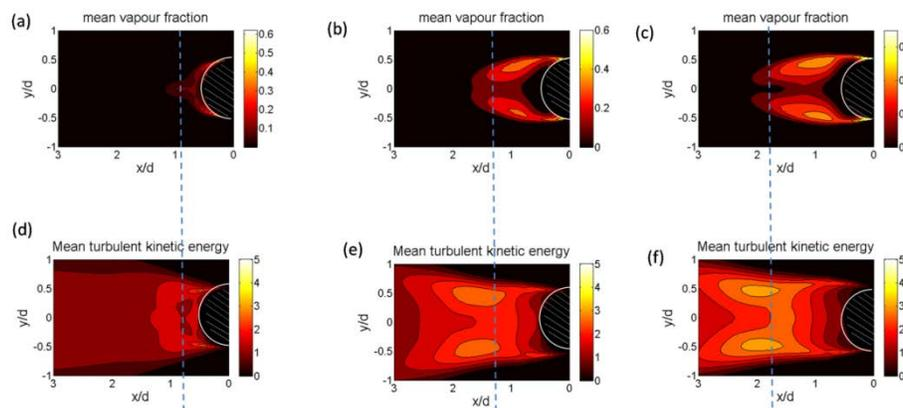
Figure 4: Mean contour of turbulent kinetic energy and vapour fraction shown for different cavitation number ( $\sigma/\sigma_v$ ): (a, d) 0.85, (b, e) 0.54, (c, f) 0.5. Dashed vertical lines shows the position of cavity collapse as well peak of turbulent kinetic energy.
