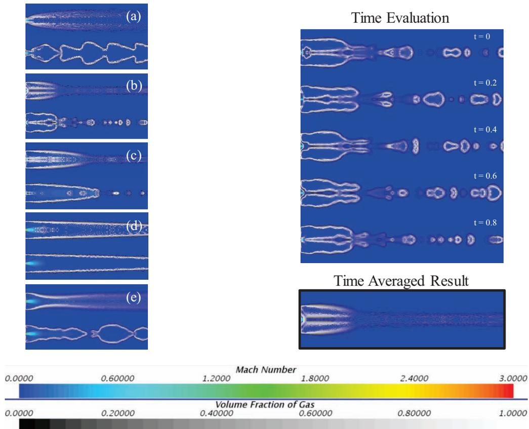
Figure 3: (a) Shedding Jet, (b) Toroidal Cavity, (c) Pulsating Cavity, (d) Stable Cavity, (e) Over-Ventilated Cavity
