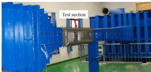
Figure 1 The high speed cavitation tunnel in CSSRC.
