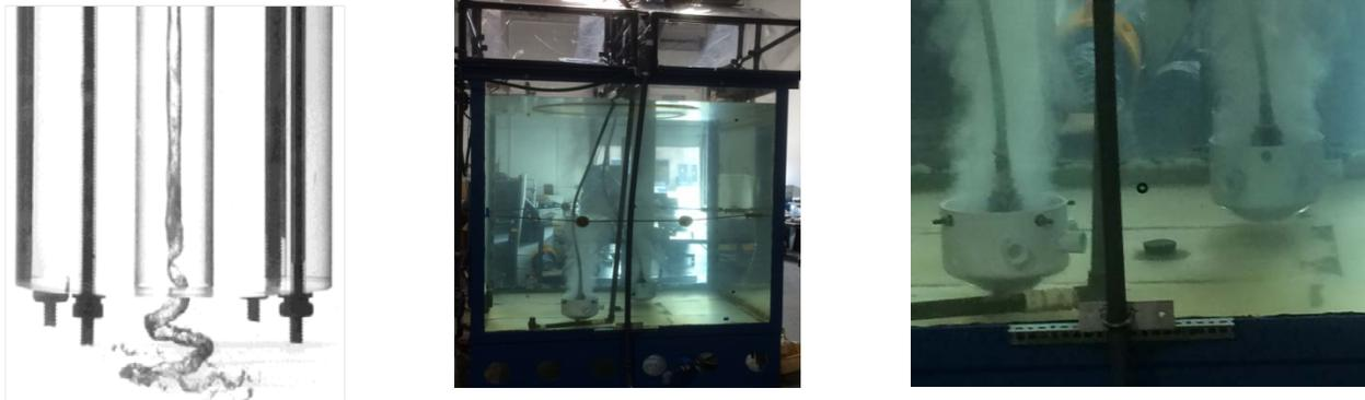
Figure 1. Cavitation Core from DYNASWIRL<sup>®</sup> nozzle (left hand photo). Large (1,350 gallon) test tank with 2 bubble generators (center hand photo). Close-up of the generators at the bottom of the tank (right hand photo).
