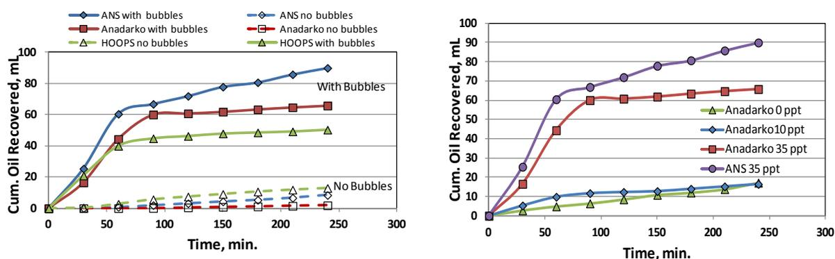
**Figure 5. (Left) Comparison of cumulative oil recovery during laboratory experiments with (solid lines) and without (dashed lines) microbubble injection for three types of crude oil: Anadarko, ANS, and HOOP all at  $\sim 0.002\%$ . (Right) Oil recovery of Anadarko at three salinity levels and ANS at 35 ppt salinity.**
