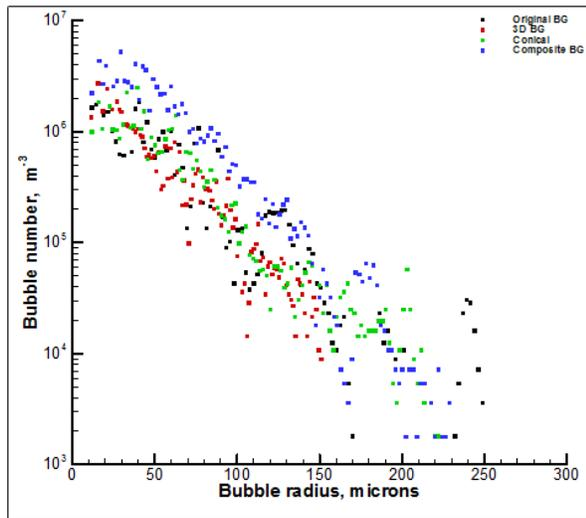
Figure 3. Bubble size distribution from nine different DYNASWIRL<sup>®</sup> bubble generators. Pump pressure 15 psi, water flow rate 26.5lpm, and air flow rate 0.46 lpm.
