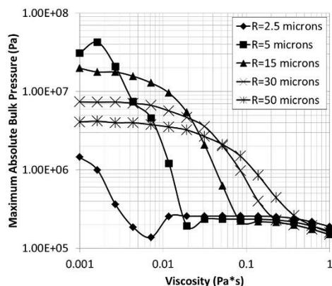
Figure 4: Maximum bulk pressure vs. viscosity.
