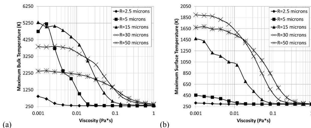
Figure 3: (a) Maximum bulk temperature vs. viscosity, and (b) maximum surface temperature vs. viscosity.
