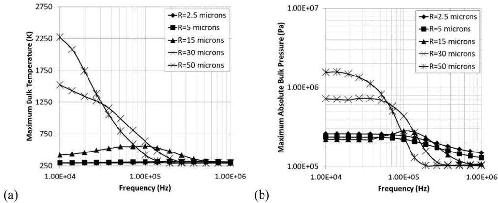
Figure 1: (a) Maximum bulk temperature vs. frequency, and (b) maximum bulk pressure vs. frequency.
