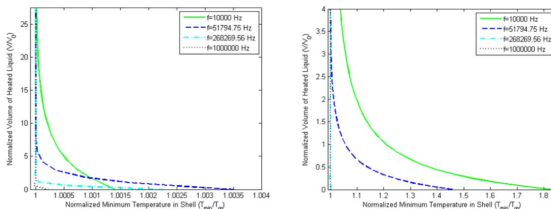
Figure 5: Dimensionless liquid volume heated vs. minimum dimensionless temperature at instant of minimum bubble volume with varying frequency. Left:  $R_0 = 5$  microns. Right:  $R_0 = 30$  microns.
