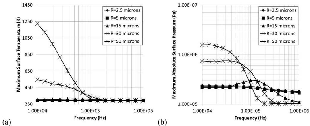
Figure 2: (a) Maximum surface temperature vs. frequency, and (b) maximum surface pressure vs. frequency.
