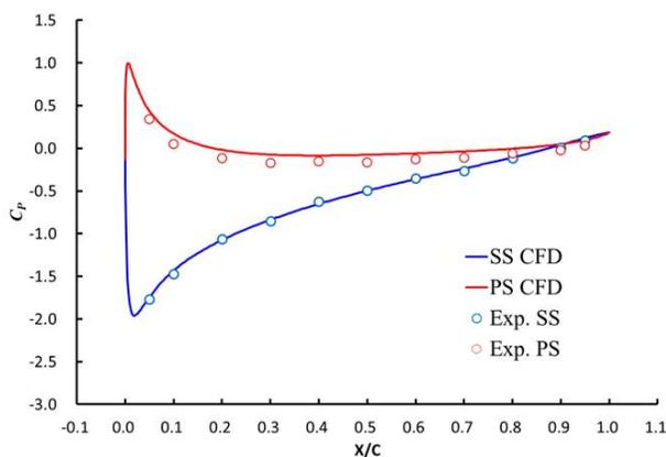
Figure 1(a) Angle of Attack 6 deg
