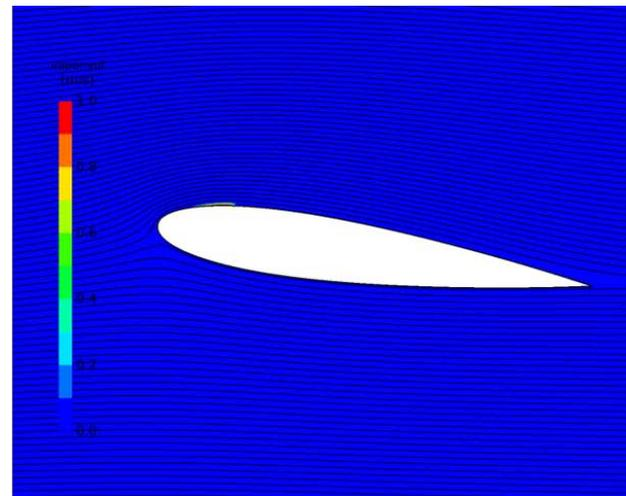
Figure 4(b) Cavi. Model with Laminar B.L.
