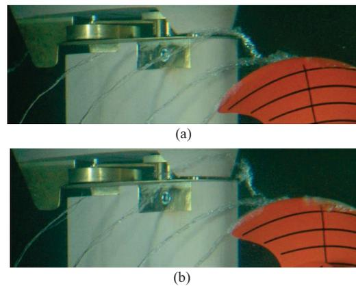
Figure 6. Collapsing of TVC at the gap between the rudder and the headbox in experiment at (a)  $\phi=350^\circ$  and (b)  $\phi=0^\circ$
